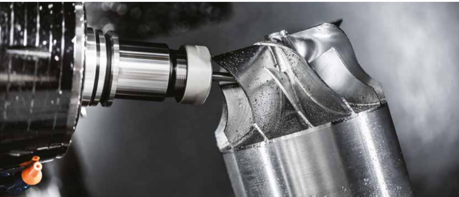
High power electro spindles have many machine tool applications including Milling, Drilling, Engraving and Routing.
